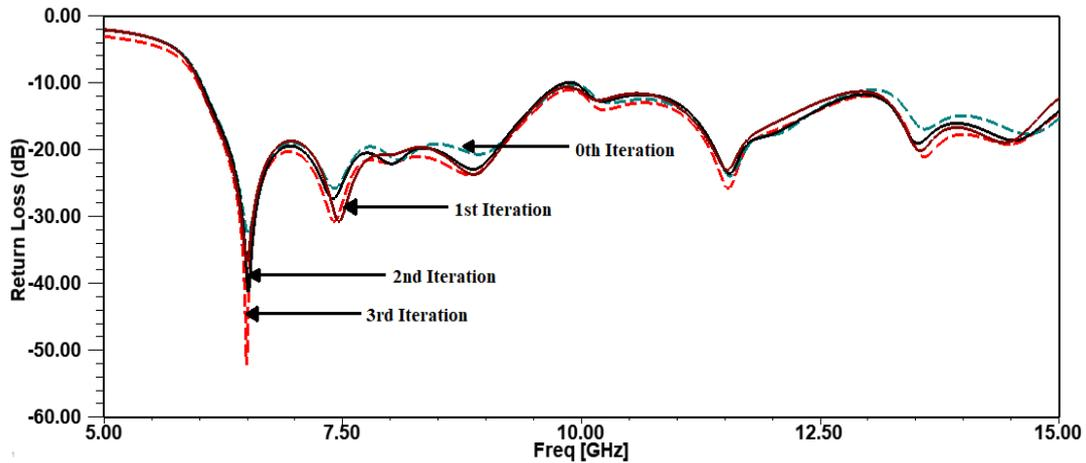
fig. 7 return loss for the repeated shape(fractals)
