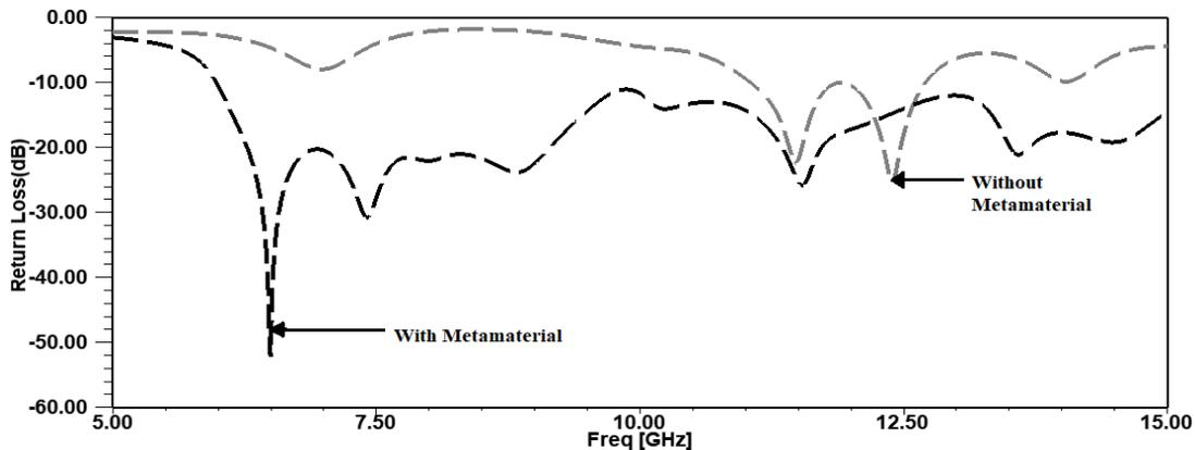
fig 8 return losses with and without the metamaterial
