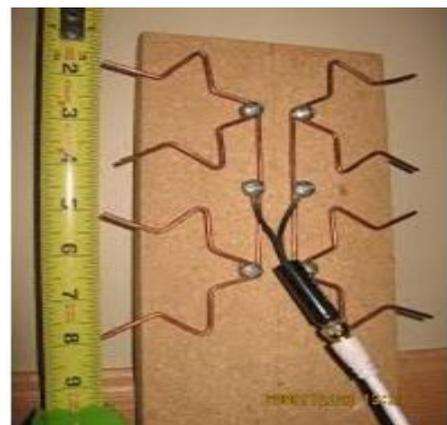
Fig.3 fractal antenna tree
