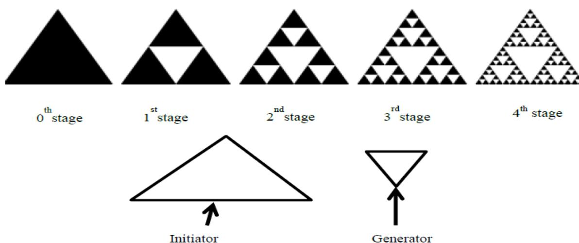
Fig. 1 different stages of fractal antenna
